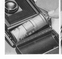
When inserting the spool, the trimmed end of the backing should point towards the empty take-up spool.
