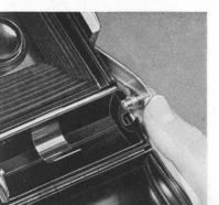
Swing out the spool holder of the lower spool chamber.
