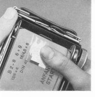
Push the backing paper sideways on the take-up spool if necessary, to make sure that it winds up straight and light-tight between the spool flanges.
